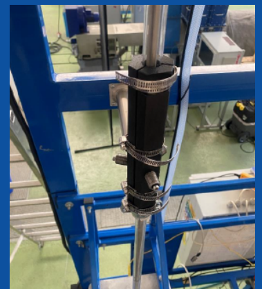
Fig. 5 Assembled Flow Channel
