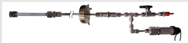
Fig. 2: Sample (left) before burst test (a valve can be seen at the top right)
