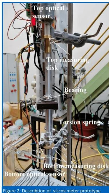
Figure 2: Description of viscosimeter prototype
