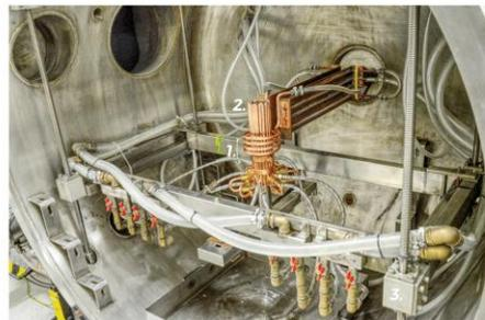
Induction system with cold crucible; 1 – inductor, 2 – cold crucible, 3 – moving device
