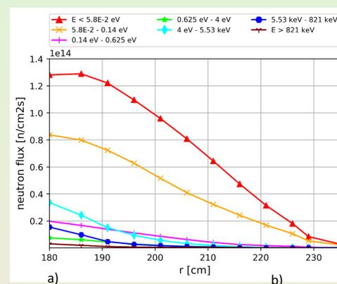
Figure 2: Radial neutron flux, detector in the middle of the fuel assembly height under the moderator level
