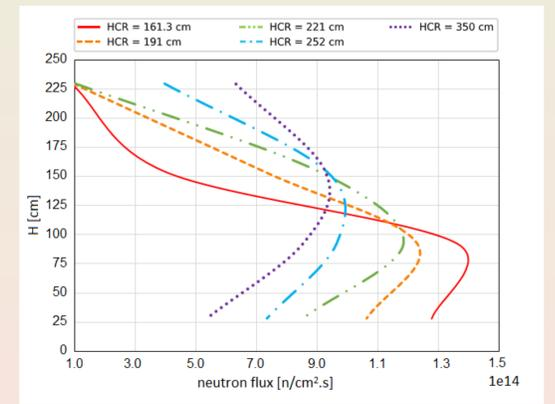
Figure 5: Effect of the moderator level on axial neutron flux profile distribution 1.group thermal neutrons
