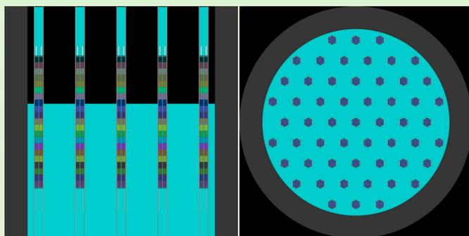
Figure 1: The model of TEPLATOR core – a) side view, b) view from above
