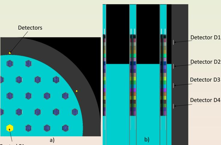
Figure 3: a) 60° symmetry of the detectors b) Axial position of the ex-core detectors
